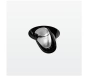
Recessed, flush with ceiling with LED, rated life of the LED L80/B10 > 50000 h, colour rendering index CRI > 80, chromaticity tolerance 2 SDCM (initial), reflector with asymmetrical light distribution pattern, primary reflector and kick reflector 99% pure aluminium in MIRO-Silver®, attachment with kick reflector for light cone projection, exchangeable reflector unit in high-sheen black plastic, with glass cover, luminaire head designed as heat sink die-cast aluminium, black anodized
