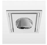
Recessed luminaire with LED, rated life of the LED L80/B10 > 50000 h, colour rendering index CRI > 80, chromaticity tolerance 3 SDCM (initial), reflector with circular light distribution pattern, swivel angle 30° luminaire housing sheet steel, powder-coated, white, separate driver unit
