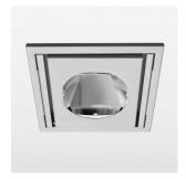
Recessed luminaire with LED, rated life of the LED L80/B10 > 50000 h, colour rendering index CRI > 90, chromaticity tolerance 2 SDCM (initial), reflector with circular light distribution pattern, swivel angle 30° luminaire housing sheet steel, powder-coated, silver, separate driver unit
