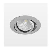
Recessed luminaire with LED, rated life of the LED L80/B10 50000 h (tambient 25°C), colour rendering index CRI > 90, chromaticity tolerance 2 SDCM (initial), reflector with circular light distribution pattern, reflector pure aluminium 99,99% in MIRO-Silver®, segmented and faceted, 3D lens silicon to reduce the proportion of scattered light, die-cast aluminium, powder-coated, rotation angle, swivel angle +/- 25°, silver,
