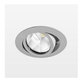
Recessed luminaire with LED, rated life of the LED L80/B10 50000 h (tambient 25°C), colour rendering index CRI > 90, chromaticity tolerance 2 SDCM (initial), reflector with oval light distribution pattern, reflector pure aluminium 99,99% in MIRO-Silver®, segmented, die-cast aluminium, powdercoated, rotation angle, swivel angle +/- 25°, silver,
