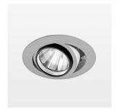
Recessed luminaire with LED, rated life of the LED L80/B10 50000 h (tambient 25°C), colour rendering index CRI > 96, chromaticity tolerance 2 SDCM (initial), rotation-symmetrical reflector with circular light distribution pattern, reflector pure aluminium 99,99% in MIRO-Silver®, segmented and faceted, 3D lens silicon to reduce the proportion of scattered light, die-cast aluminium, powder-coated, rotation angle, swivel angle +/- 25°, silver,
