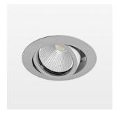
Recessed luminaire with LED, rated life of the LED L80/B10 50000 h (tambient 25°C), colour rendering index CRI > 90, chromaticity tolerance 2 SDCM (initial), reflector with circular light distribution pattern, reflector pure aluminium 99,99% in MIRO-Silver®, segmented and faceted, die-cast aluminium, powder-coated, rotation angle, swivel angle +/- 25°, silver,
