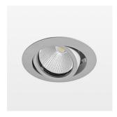
Recessed luminaire with LED, rated life of the LED L80/B10 50000 h (tambient 25°C), colour rendering index CRI > 96, chromaticity tolerance 2 SDCM (initial), reflector with circular light distribution pattern, reflector pure aluminium 99,99% in MIRO-Silver®, segmented and faceted, 3D lens silicon to reduce the proportion of scattered light, die-cast aluminium, powder-coated, rotation angle, swivel angle +/-  $25^{\circ}$ , silver,
