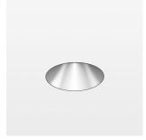
Recessed downlight, flush with ceiling with LED, rated life of the LED L80/B10 > 50000 h, colour rendering index CRI > 96, chromaticity tolerance 2 SDCM (initial), reflector with homogeneous light distribution pattern, diffuser lens, translucent, darklight reflector, aluminium, metallised, highgloss, luminaire head die-cast aluminium,
