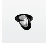
Recessed, flush with ceiling with LED, rated life of the LED L80/B10 > 50000 h, colour rendering index CRI > 70, chromaticity tolerance 2 SDCM (initial), reflector with asymmetrical light distribution pattern, primary reflector and kick reflector 99% pure aluminium in MIRO-Silver®, attachment with kick reflector for light cone projection, exchangeable reflector unit in high-sheen black plastic, with glass cover, luminaire head designed as heat sink die-cast aluminium, black anodized
