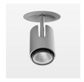
Semi-recessed luminaire with LED, rated life of the LED L80/B10 50000 h (tambient 25°C), colour rendering index CRI > 95, chromaticity tolerance 2 SDCM (initial), reflector with circular light distribution pattern, reflector pure aluminium 99,99% in MIRO-Silver®, segmented and faceted, exchangeable reflector unit in high-sheen black plastic, with glass cover, rotation angle 330°, swivel angle +/- 90°; luminaire housing die-cast aluminium, powder-coated, silver, separate driver unit
