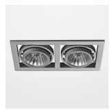
Recessed luminaire with LED, rated life of the LED L80/B10 > 50000 h, colour rendering index CRI > 90, chromaticity tolerance 2 SDCM (initial), reflector with circular light distribution pattern, swivel angle  $\pm$  30° luminaire housing sheet steel, powder-coated, silver, separate driver unit
