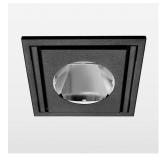
Recessed luminaire with LED, rated life of the LED L80/B10 > 50000 h, colour rendering index CRI > 80, chromaticity tolerance 3 SDCM (initial), reflector with circular light distribution pattern, reflector pure aluminium 99,99% in MIRO-Silver®,, swivel angle 30° luminaire housing sheet steel, powder-coated, black, separate driver unit
