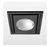
Recessed luminaire with LED, rated life of the LED L80/B10 > 50000 h, colour rendering index CRI > 70, chromaticity tolerance 2 SDCM (initial), reflector with oval light distribution pattern, swivel angle  $30^{\circ}$  luminaire housing sheet steel, powder-coated, black, separate driver unit
