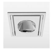
Recessed luminaire with LED, rated life of the LED L80/B10 > 50000 h, colour rendering index CRI > 90, chromaticity tolerance 2 SDCM (initial), reflector with circular light distribution pattern, swivel angle 30° luminaire housing sheet steel, powder-coated, white, separate driver unit
