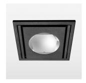
Recessed luminaire with LED, rated life of the LED L80/B10 > 50000 h, colour rendering index CRI > 90, chromaticity tolerance 2 SDCM (initial), reflector with oval light distribution pattern, swivel angle 30° luminaire housing sheet steel, powder-coated, black, separate driver unit
