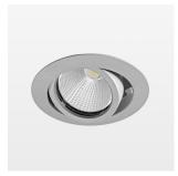
Recessed luminaire with LED, rated life of the LED L80/B10 50000 h (tambient 25°C), colour rendering index CRI > 90, chromaticity tolerance 2 SDCM (initial), reflector with circular light distribution pattern, reflector pure aluminium 99,99% in MIRO-Silver®, segmented and faceted, 3D lens silicon to reduce the proportion of scattered light, die-cast aluminium, powder-coated, rotation angle, swivel angle +/-  $25^{\circ}$ , silver,
