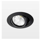
Recessed luminaire with LED, rated life of the LED L80/B10 50000 h (tambient 25°C), colour rendering index CRI > 80, chromaticity tolerance 2 SDCM (initial), reflector with oval light distribution pattern, reflector pure aluminium 99,99% in MIRO-Silver®, segmented, die-cast aluminium, powdercoated, rotation angle, swivel angle +/- 25°, black,
