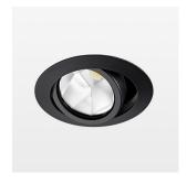
Recessed luminaire with LED, rated life of the LED L80/B10 50000 h (tambient 25°C), colour rendering index CRI > 96, chromaticity tolerance 2 SDCM (initial), reflector with oval light distribution pattern, reflector pure aluminium 99,99% in MIRO-Silver®, segmented, die-cast aluminium, powder-coated, rotation angle, swivel angle +/- 25°, black,
