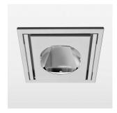
Recessed luminaire with LED, rated life of the LED L80/B10 > 50000 h, colour rendering index CRI > 80, chromaticity tolerance 3 SDCM (initial), reflector with circular light distribution pattern, swivel angle 30° luminaire housing sheet steel, powder-coated, silver, separate driver unit
