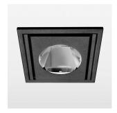
Recessed luminaire with LED, rated life of the LED L80/B10 > 50000 h, colour rendering index CRI > 80, chromaticity tolerance 3 SDCM (initial), reflector with circular light distribution pattern, swivel angle 30° luminaire housing sheet steel, powder-coated, black, separate driver unit
