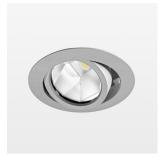
Recessed luminaire with LED, rated life of the LED L80/B10 50000 h (tambient 25°C), colour rendering index CRI > 96, chromaticity tolerance 2 SDCM (initial), reflector with oval light distribution pattern, reflector pure aluminium 99,99% in MIRO-Silver®, segmented, die-cast aluminium, powdercoated, rotation angle, swivel angle +/- 25°, silver,
