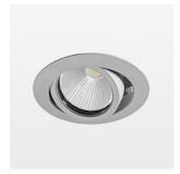
Recessed luminaire with LED, rated life of the LED L80/B10 50000 h (tambient 25°C), colour rendering index CRI > 80, chromaticity tolerance 2 SDCM (initial), reflector with circular light distribution pattern, reflector pure aluminium 99,99% in MIRO-Silver®, segmented and faceted, 3D lens silicon to reduce the proportion of scattered light, die-cast aluminium, powder-coated, rotation angle, swivel angle +/- 25°, silver,
